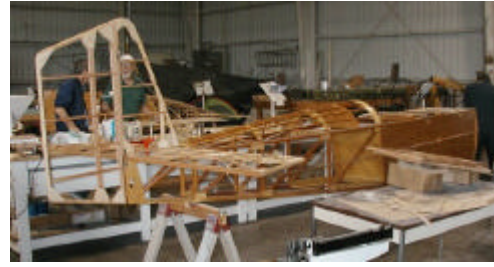
The Pietenpol takes shape as the turtle deck is now glued in place
