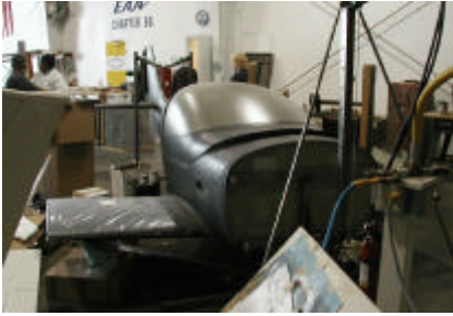
The front view with rotisserie to "flip" fuselage to work on the bottom panels. If you are doing a composite aircraft, you must
