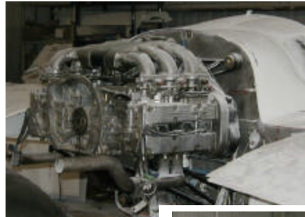
The Cozy-IV is back on its gear with the 6-cyl Subaru mounted to the rear firewall
